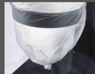
Dust separation in Longbag
